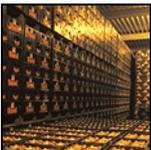
Secondary fermentation occurs at 22 °C for 10 days. After the warm comes the cold cell, where the beer stays for 6 weeks at a temperature of 6 °C.
