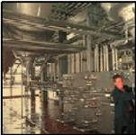
High fermentation takes place at a temperature of 20 to 26 °C for 4 to 8 days. Then, the beer is cooled to 0 °C for 3 weeks in conditioning vats for maturation. Every 15 minutes, the fermentation temperature is captured.
