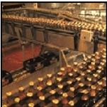
Barrels or bottles are filled with the beer after they have been cleaned and sterilised. Pressure and temperature are monitored. Recipe & best before date are major lot ID parameters.
